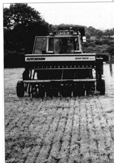
Specialist direct drills like this Aitchison Seedmatic from New Zealand have performed best in over-seeding establishment trials.
