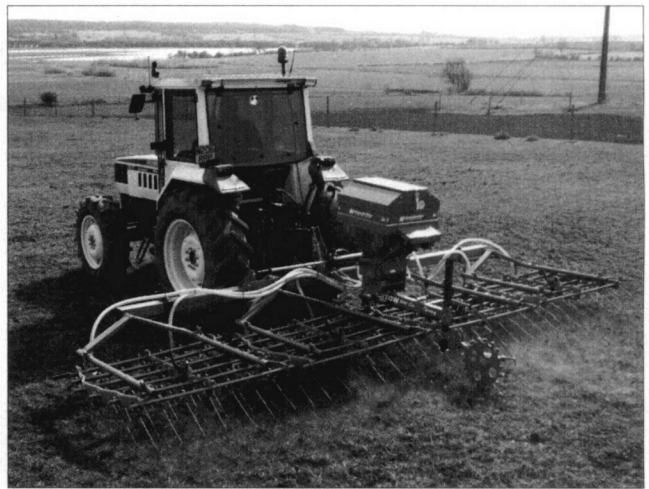
Tine harrow seeders like this Opico Hatzenbichler have a work rate advantage and are widely used for general grass grooming operations.
